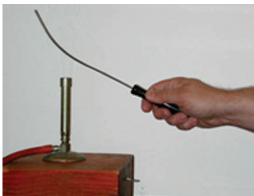
Sumber: www.physics.upenn.edu Gambar 4.6 Saat dipanaskan, bimetal melengkung.
